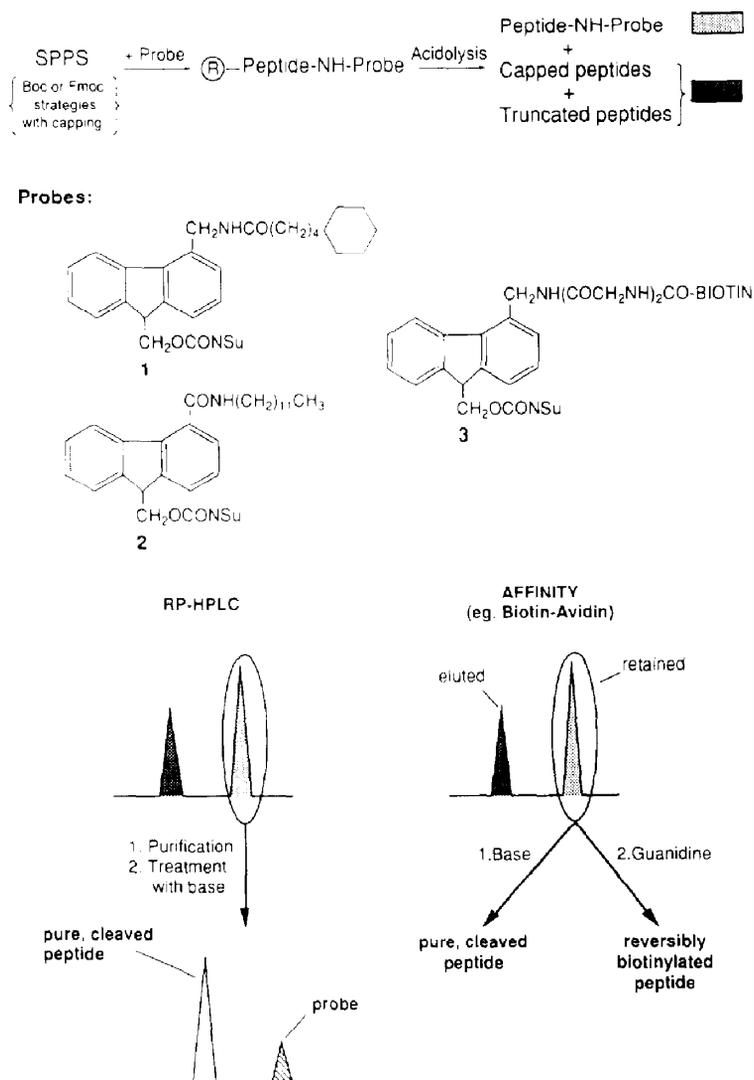
Fig. 1. General scheme showing application of chromatographic probes 1, 2 and 3.
