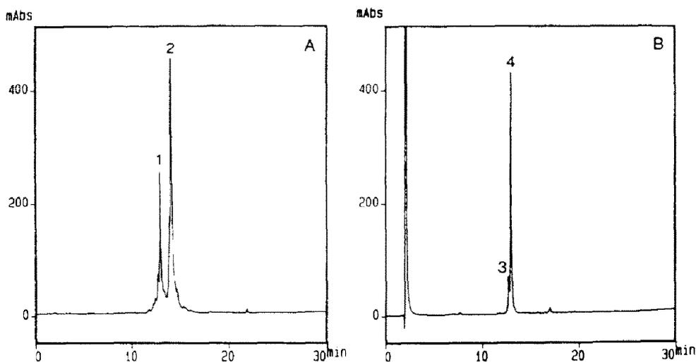
Fig. 5. Analytical RP-HPLC on a Vydac  $C_{18}$  column ( $150 \times 4.6$  mm I.D.) connected to a Shimadzu LC10 LC system. Solvent A, water–0.045% TFA; solvent B, acetonitrile–0.036% TFA; gradient, 0–100% B in 30 min; flow-rate, 1 ml/min; detection, 20 nm. (A) Crude  $\beta$ 2-subunit adduct + **3**; (B) purified  $\beta$ 2-subunit after elution from immobilized avidin with base.
