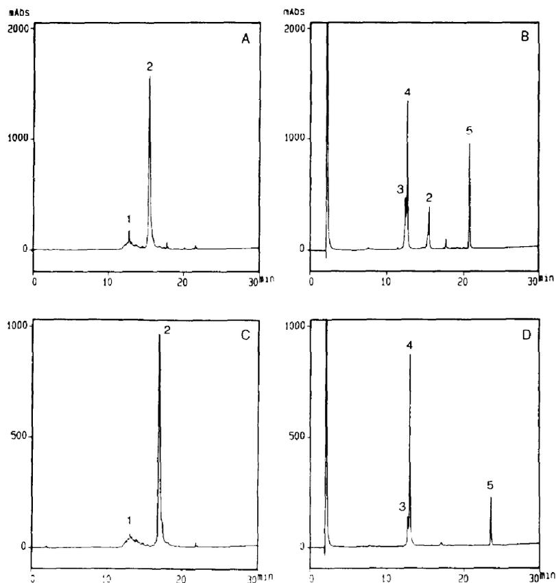
Fig. 2. Analytical RP-HPLC on a Vydac  $C_4$  column ( $150 \times 4.6$  mm I.D.) connected to a Shimadzu LC10 LC system. Solvent A, water–0.045% TFA; solvent B, acetonitrile–0.036% TFA; gradient, 0–100% B in 30 min; flow-rate, 1 ml/min; detection, 220 nm. (A) Crude  $\beta$ 2-subunit adduct + 1; (B) purified  $\beta$ 2 subunit adduct + 1; (C) crude  $\beta$ 2-subunit adduct + 2; (D) purified  $\beta$ 2-subunit adduct + 2.
